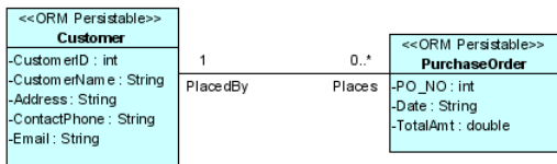
Figure 17.29 - Class Diagram with association and multiplicity
