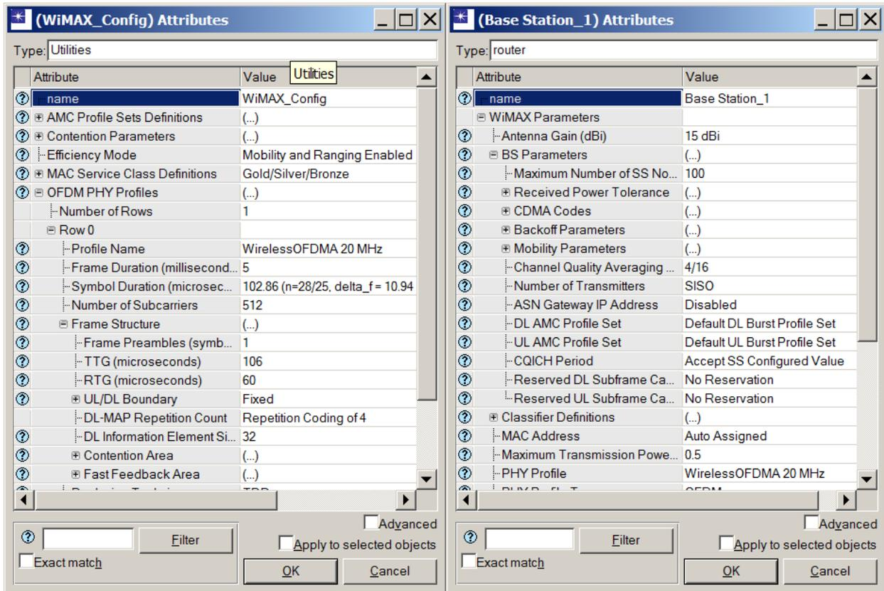
Figure 3. Configuration parameters for QPSK scenario: WiMAX\_Config and base station.
