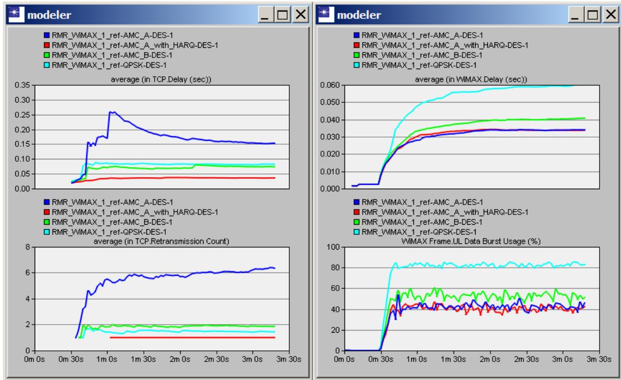
Figure 10. Simulation results for scenario AMCA\_with\_HARQ versus AMCA, AMCB, and QPSK.
