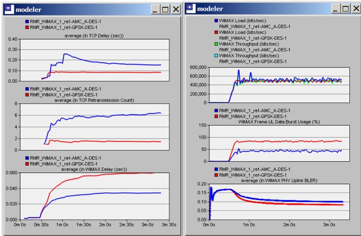
Figure 7. Simulation results for the scenario AMC\_A versus the scenario QPSK.
