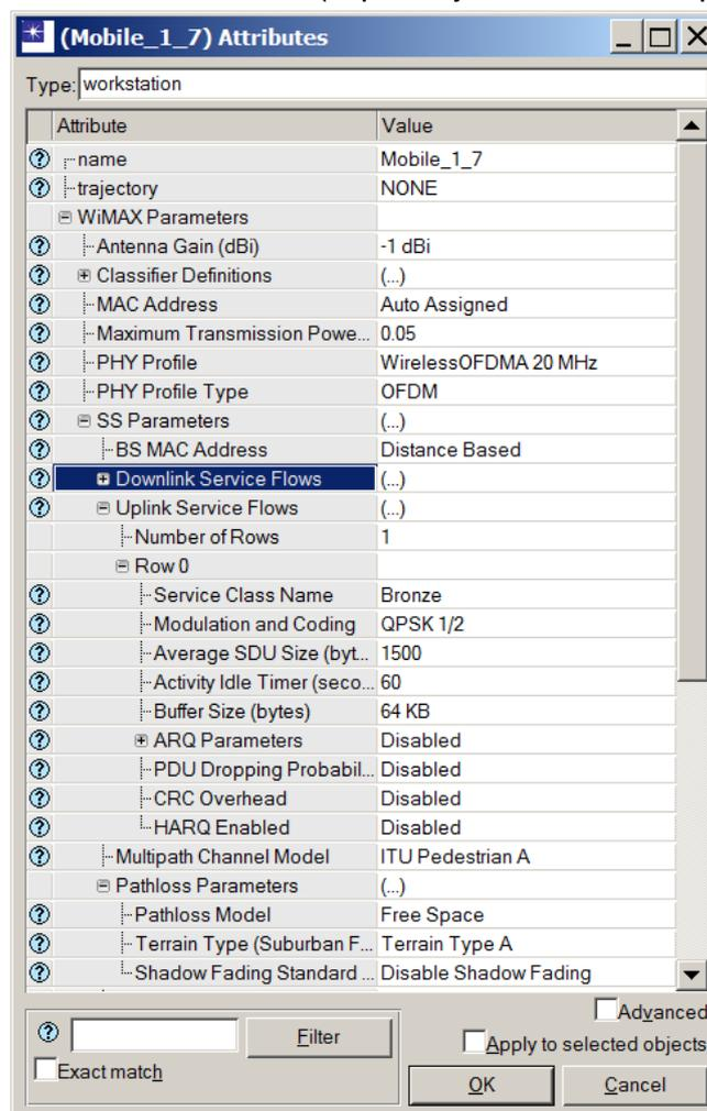
Figure 2. Configuration parameters for QPSK scenario: subscriber (mobile) stations.
